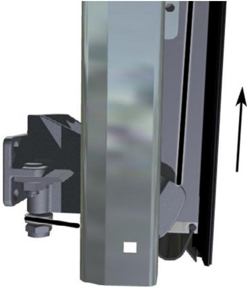
When using an electric operated door a microswitch (article number: 25446A) needs to be installed on the cable break device. The rotation of the rotating module will cut the power to the motor, preventing the operator to cause damages.
