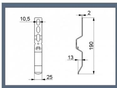
Installation bracket for connecting the lintel profile against the wall or ceiling.
