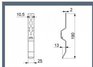
Installation bracket for connecting the lintel profile against the wall or ceiling.
