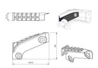
This top-curve roller position displacer optimizes the closing position of the top roller and secures the top panel more tightly against the side and top sealing.
