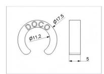
Able to put on rollers after installation. Suitable for 11mm rollers. Thickness 5mm. Color similar to RAL 9006.
